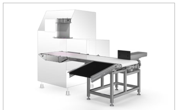
Core segment inspects large, chunky products
